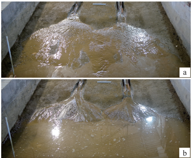
图7 性质不同的流体的沉积过程(图中白尺长30 cm) (a)重力流沉积过程;(b)牵引流改造过程 Fig.7 Deposition process of fluids with different properties (the length of white ruler is 30 cm) (a) deposition process of gravity flow; (b) modification process of the traction current
